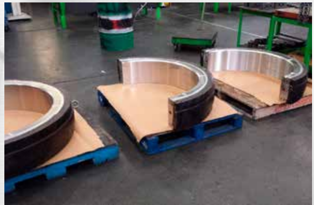
Refurbished Mill bearings
